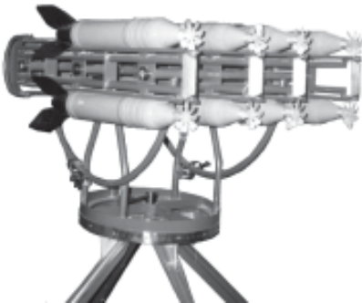
Fig. 13.7. Katyusha 's little sister: smaller 3.3-in. (82-mm) rockets M-8 developed by the USSR during World War II. The mobile launcher, called Stalin Organ , could fire 30 to 48 such 17.5-lb (8-kg) rockets to a distance of up to 3 miles (4.8 km). A later missile model had mass 31 lb (14 kg) and a larger range. Photo courtesy of Mike Gruntman.
