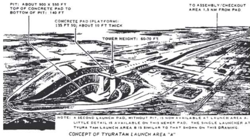
Fig. 14.21. Top: one of the first U-2 photographs of the Tyuratam launching pad in 1950s. The first ICBM, the first satellite, and the first cosmonaut were launched from this site. Bottom: sketch of this launching site in 1961 based on U-2 and Corona satellite photographs. Figures courtesy of Central Intelligence Agency.
