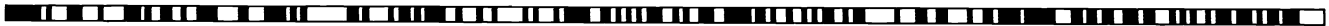
Fig.8. The coded-aperture basic sequence generated by the primitive polynomial h(x) = x^8 + x^6 + x^5 + x^1 + 1 .
