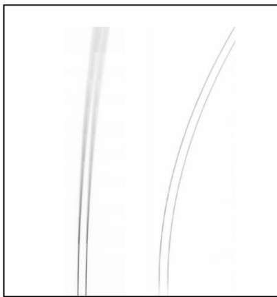
Figure 4 (above): Sodium doublet spectrum CCD images taken with a single straight slit (left) vs. single curved slit (right). Doublet wavelengths are 589.0 and 589.6 nm.
