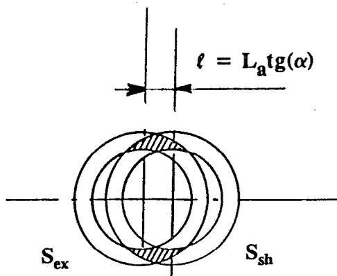
FIG. 2. "Shadow" cast by the entrance annular slit on the plate of the exit slit;  $S_{ex}$  is the exit slit and  $S_{sh}$  is the shadow of the entrance slit. The hatched area corresponds to the effective area (in the absence of the deflecting plates) of the collimator transmitting ENAs coming from the off-axis angle  $\alpha$ .
