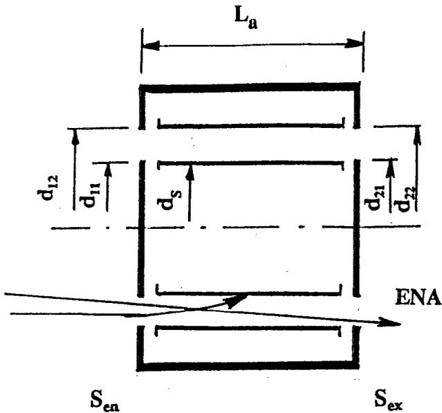
FIG. 1. Axis-symmetric annular collimator with the identical entrance and exit slits;  $S_{en}$  is the entrance slit and  $S_{ex}$  is the exit slit. The trajectories of ENA (straight line) and ion (curved line hitting the deflector plate) are shown.
