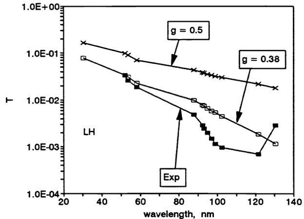
Fig.6. Spectral dependence of the transmission  $T_\Sigma = T_P + T_S$ . *Exp* curve is the experimentally determined values. Calculated dependences are shown for two different grating geometrical transparencies,  $g=0.5$  and  $g=0.38$ .
