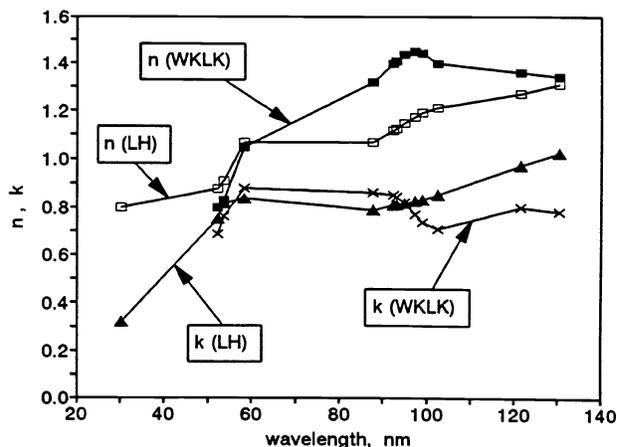
Fig.4. Spectral dependence of the index of refraction,  $n$ , and the extinction coefficient,  $k$ , for gold; WKLK<sup>19</sup> and LH.<sup>20</sup>
