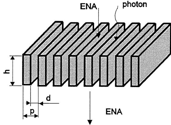
Fig.1. Schematic view of a free-standing transmission grating
