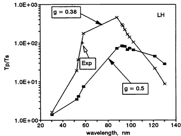
Fig.7. Spectral dependence of the transmission  $T_R = T_P/T_S$ . *Exp* is the experimentally determined value at 58.4 nm. Calculated dependences are shown for two different grating geometrical transparencies,  $g=0.5$  and  $g=0.38$ .
