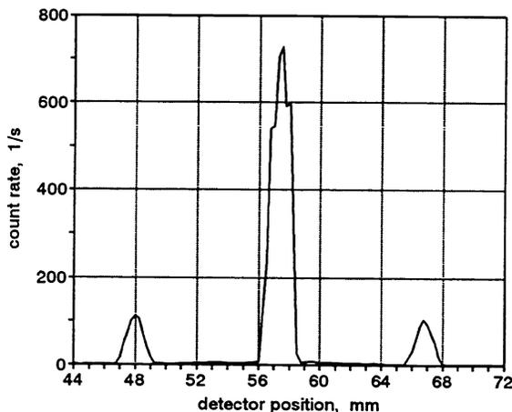
Fig.8. Detector count rate as a function of the distance from the axis (diffraction angle);  $\lambda = 58.4$  nm; WKLK<sup>19</sup> and LH.<sup>20</sup>
