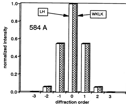
Fig.9. Calculated radiation intensity distributions across diffraction maxima;  $\lambda = 58.4$  nm; WKLK<sup>19</sup> and LH.<sup>20</sup>
