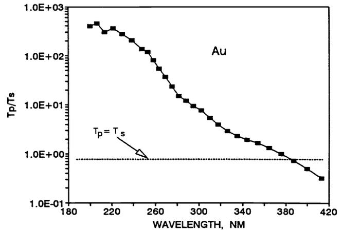
Fig.9. Calculated spectral dependence of the ratio of transmissions,  $T_R=T_P/T_S$ . Grating material is gold; grating period,  $p=500$  nm; geometrical transparency,  $g=0.4$ ; and length,  $h=1000$  nm
